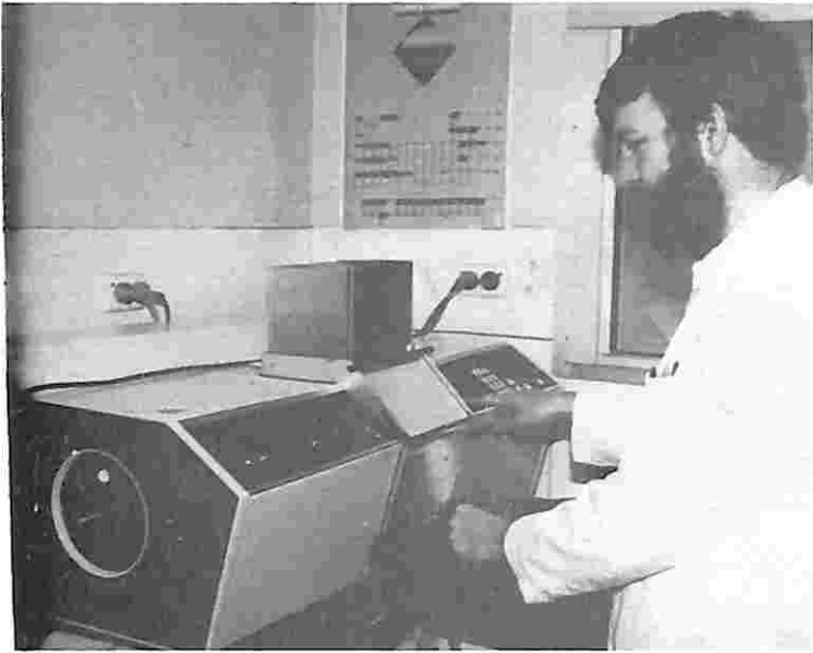
Scientist, Mr Graham Exell, measures trace metals in blood using the atomic absorption spectrophotometer purchased by the hospital.
